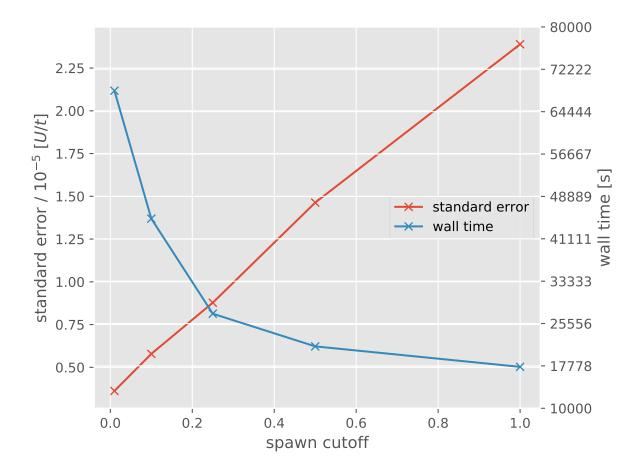
For convenience, the integer amplitude calculation is shown as having a spawn\_cutoff of 1. Clearly there is a playoff between the computational cost and the desired stochastic error; choosing a value of 0.25 for spawn\_cutoff in this case seems sensible as it is around the point where the rate of change in the wall time begins to slow<sup>4</sup>.
