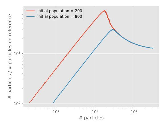
We see that the calculation with a larger initial population has a shoulder at a larger number of particles, effectively overshooting the shoulder. At yet larger numbers of particles than this, we expect the calculation to be stable once population control is enabled (i.e. the shift is allowed to vary).
