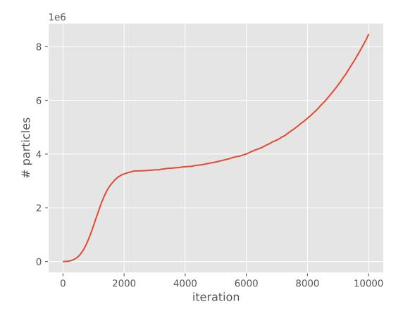
systems with a small Hilbert space) or appear as a shoulder (common in CCMC calculations). *pyhande* contains two algorithms for determining the plateau, which are helpful in such cases or for automatically analysing large numbers of calculations.
