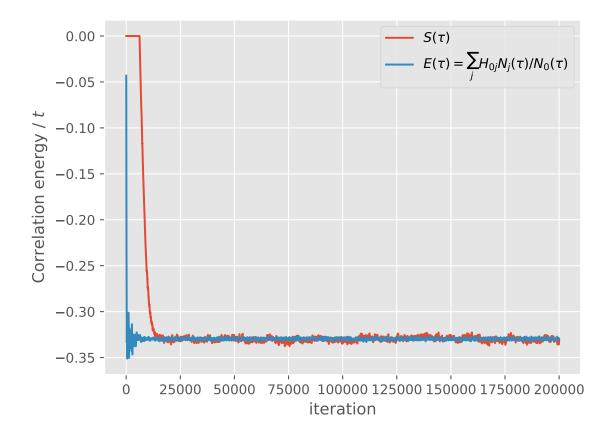
The stochastic error can be reduced by running with more particles and/or running for longer. Another very effective method is to allow determinants to have fractional numbers of particles on determinants rather than just using a strictly integer representation of the wavefunction. This is done using the real\_amplitudes keyword:
